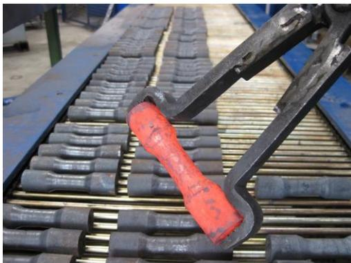
Forged preforms created by using cross wedge rolling must be further processed in order to obtain the final shape. (Source: IPH)
